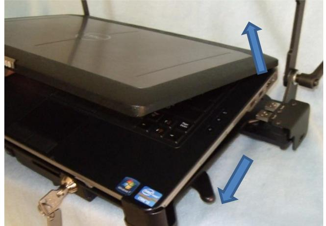
2. Ensure the handle is all the way forward, then lift the back of the laptop up and out of the dock.
