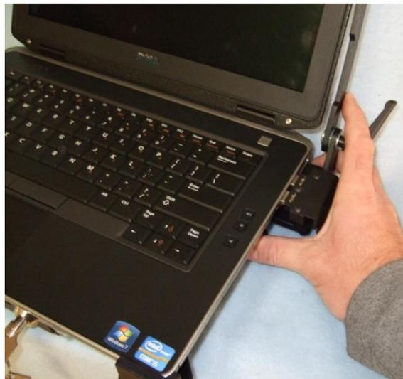
2. Now insert the laptop and carefully guide the plugs into their respective connectors. Remove the key from the dock, and retighten the screws loosened in step 1. All ports should now be aligned and ready for easy laptop docking.
