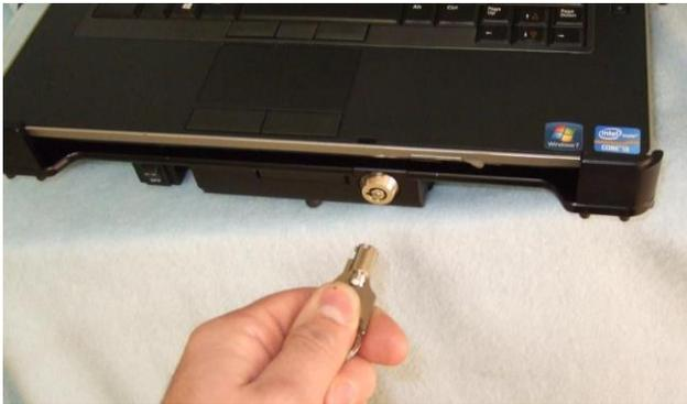
1. Insert key and turn 90 degrees counter clockwise. Springs will release the connector plugs and the handle will come forward.
