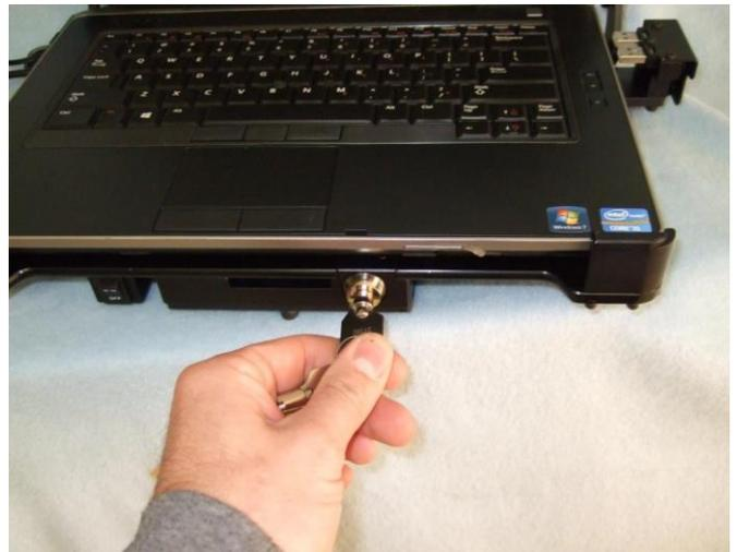
4. Pre-load the lock by turning the key 90 degrees clockwise.
