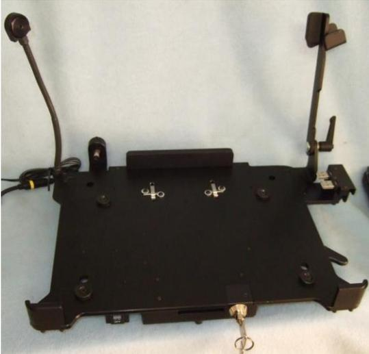
1. Prep the dock by unlocking the lock mechanism. Insert key and turn 90 degrees counter clockwise.
