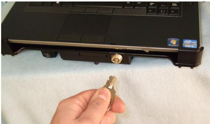
7. Once the connectors are fully engaged the key will be easily removed. Note that if the key does not come out, the laptop is not fully secure.
