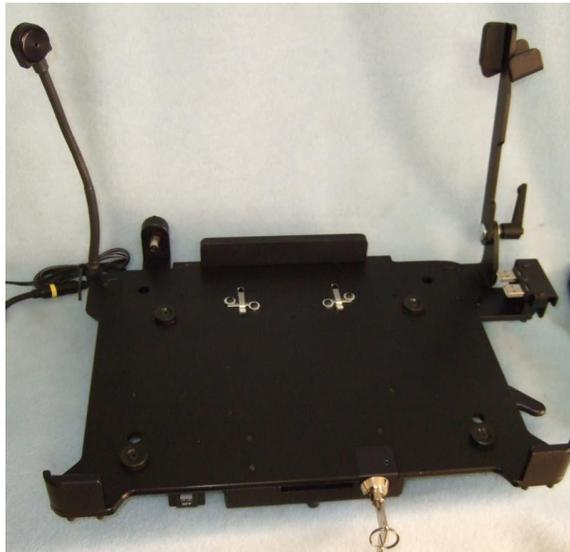
3. You can now either leave the key in it's position for quick re-insertion later, or turn the key 90 degrees clockwise, then push the handle forward to be able to remove the key.
