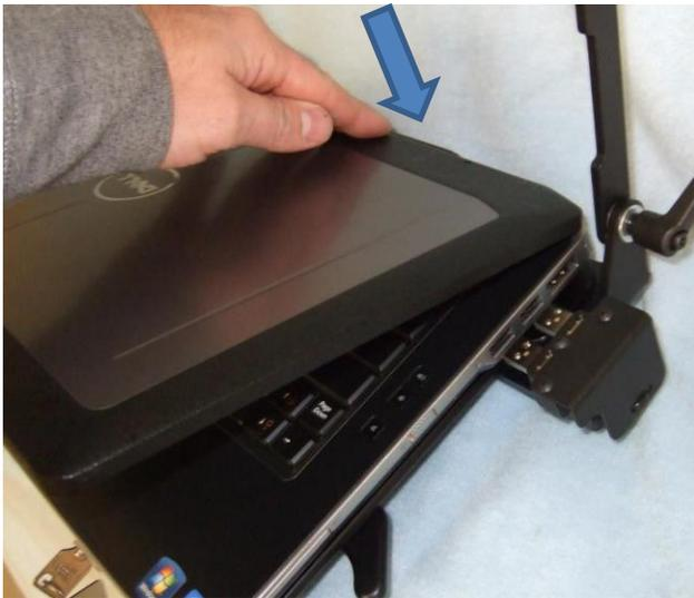
3. Press down on the back end of the laptop to ensure it is fully seated.
