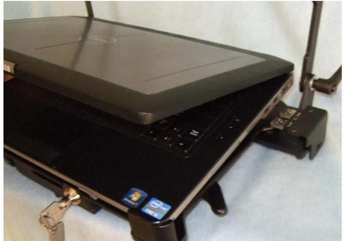
2. Open the screen of the laptop and insert the front edge into the front clamps of the dock first, then lower the back end down.
