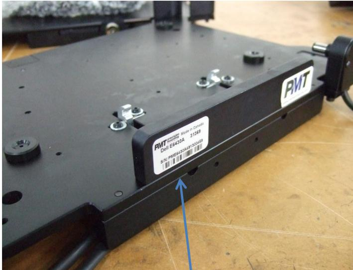
The serial number and model information label are located on the back of the vehicle dock.
