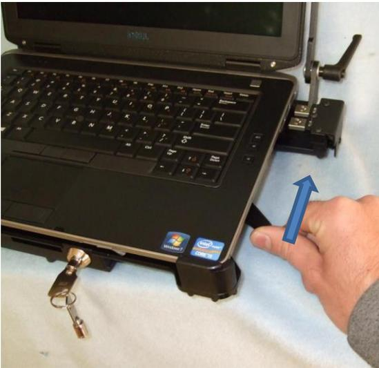
5. Drive the handle forward to engage the ports and to secure the laptop. If you feel significant resistance stop and check alignment of connectors.
