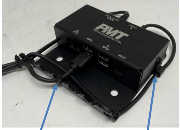
Plastic zip ties used to secure cables to Cable Tie Rail
