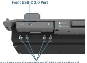
**External Antenna Connections (SMA) x4 (optional)**
