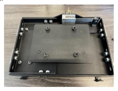
Step 2 – Place the magnet mount assembly over the nuts as shown, and use the provided M4 x 20mm screws to fasten the Magnet Mount to the Cradle. Notice use of the offset VESA holes to allow clearance from the lock module.
