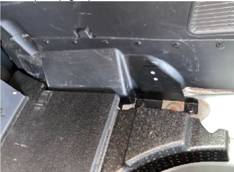
Fig.11 IMAGE SHOWN FROM REAR END PASSENGER BRACKET INSTALLED
