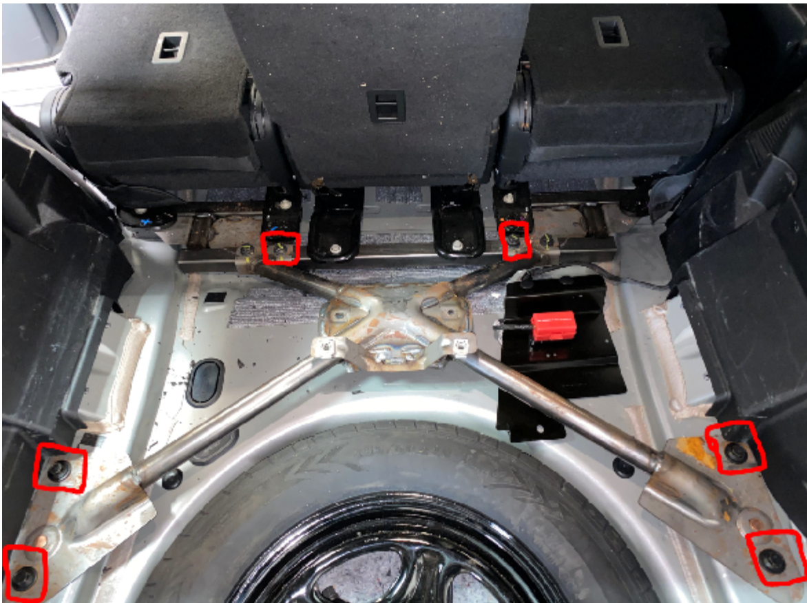
Fig.4 IMAGE SHOWING SIX OEM BOLTS NEEDED TO BE REMOVED
