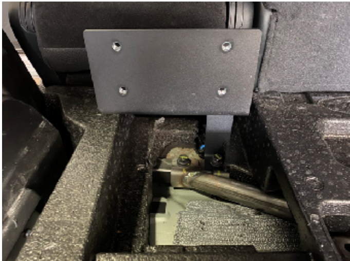
Fig.7 IMAGE FROM REAR END INSTALLED DRIVER SIDE LOWER BRACKET
