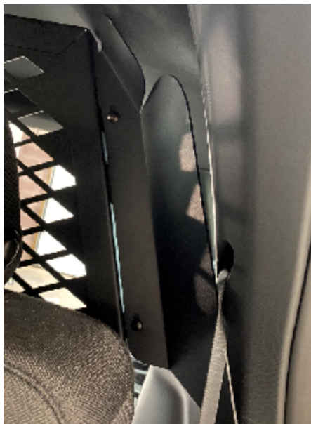
Fig.14 IMAGE DRIVER SIDE UPPER WING INSTALLED
