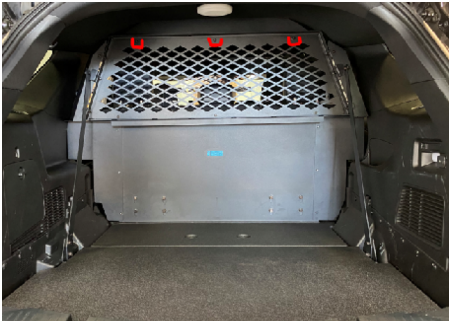
Fig.17 IMAGE SHOWN FROM REAR END PASSENGER BRACKET INSTALLED
