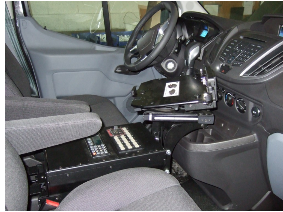
Console installed in Ford Transit with rugged laptop mounted on mouse trap motion mount
