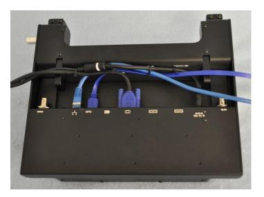
Step 1: Connect all cables securely to dock connections. Use cable ties to secure cables to the built-in cable tie slots.
