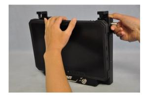
Step 2: Push docking lever up and simultaneously tilt the top of the computer forward.
