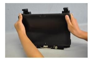
Step 3: Remove the computer by lifting it out of the dock.
