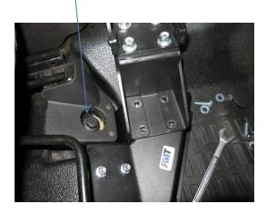
Step 5: Re-install the front seat mounting bolts and tighten to manufacturers specified torque. Re-tighten rear bolts to specified torque as well.
