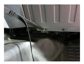
Step 8: Find a suitable location with steel bracing to hook the support straps into. Most vehicles have steel bracing behind the plastic panels under the glove box. Be sure that the area you chose to hook the straps is strong enough to support the load
