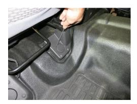
Step 1: Remove any plastic caps covering the front and rear seat mounting bolts of the front passenger seat
