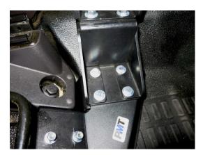
Step 6: Position the vertical pedestal, or offset riser (some vehicles may or may not require the Offset Riser) on the vehicle base and loosely thread the supplied hardware into the base. Fully tighten bolts once all four are installed
