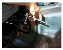
Step 2: Remove front seat mounting bolts completely
