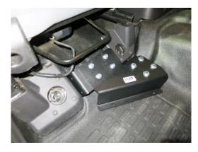
Step 4: Tilt the seat back, and slide the vehicle specific base assembly in between the vehicle floor and seat brackets. Leave any bolts present on vehicle specific base present, but loose.
