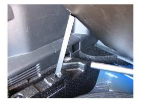
Step 5. Remove the factory center tire clamp braket
