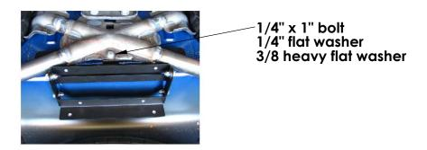
Step 4. Attaching the X-Brace Clamp: Loosely attach the X-brace clamp bracket with the (4)  $1/4 \times 5/8$ " long bolts and flat washers. Once all the bolts are started and the unit centered on the X-brace, tighten the  $1/4 \times 1$ " bolt in the center of the X-brace installed in step 3. This will pull the hinge assembly up to the X-brace to hold it centered in the vehicle. Then tighten the remaining (4) 1/4 bolts to hold the hinge mechanism in place.
