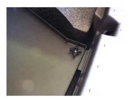
Step 3. Rotate the tray to the upward position by lifting upward on the front of the tray then rotating the back of the tray upward so it is supported by the X-brace. Step 4. The legs on the bottom of the tray are held with magnets. Pull the legs downward from the bottom of the shelf so they sit on the foam on the sides of the wheel well.
