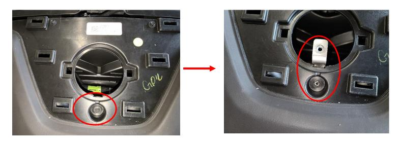
**Step 8**: Re-install the center hex bolt that was removed on step 7 and make sure it is secured and tight
