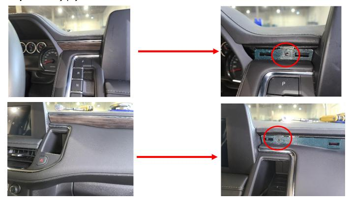
Step 2: Remove the OEM Hex head bolts on both sides
