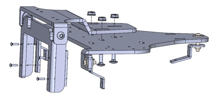
**Step 11**: Attach the Siren controller to the bracket and secure it with screws provided in the assembles
