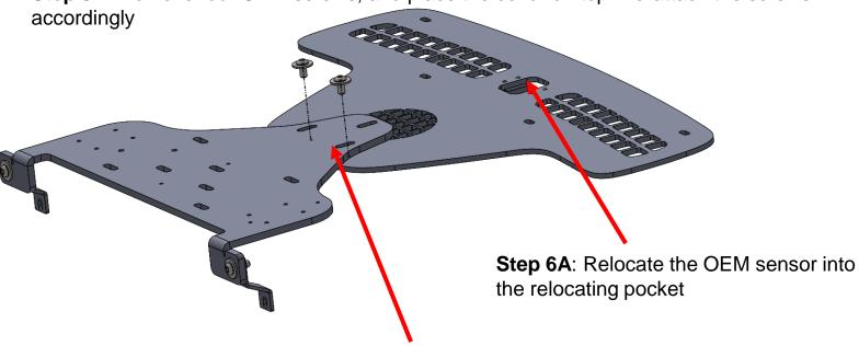
**Step 6B**: Place the dashmount base on top, and use 2x 1/4-20UNC X 1/2" screws and washers from the hardware bag and tighten both the cover and dashmount base.
