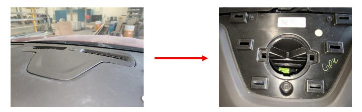
Step 6: Match the drilling template paper on top of the cover and the drill Ø 3/8" hole
