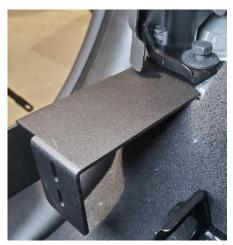
b) Place the bracket under the seat bracket and put the original bolt in place and leave it loose (both sides).
