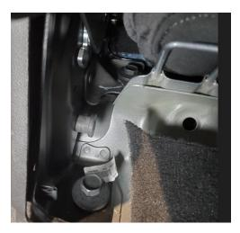
a) Uninstall the seat brackets using a proper wrench.
