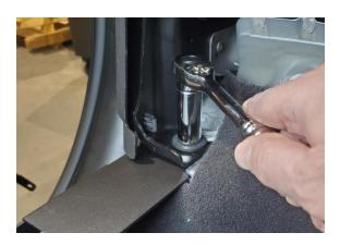
c) Tighten the original seat bracket bolts as per OEM recommended torque.
