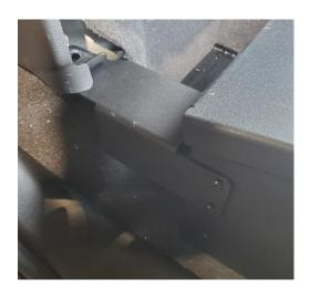
b) Fully tighten the side brackets 10-24 screws and nuts.
