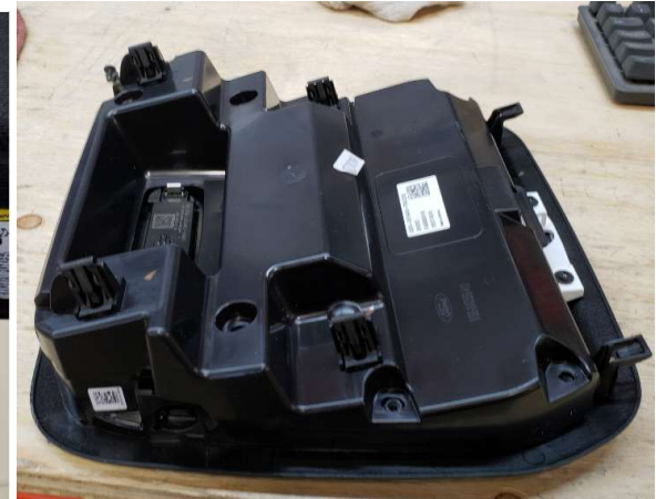
Use T-20 Torx screw driver to remove 10 T-20 screws from the back cover
