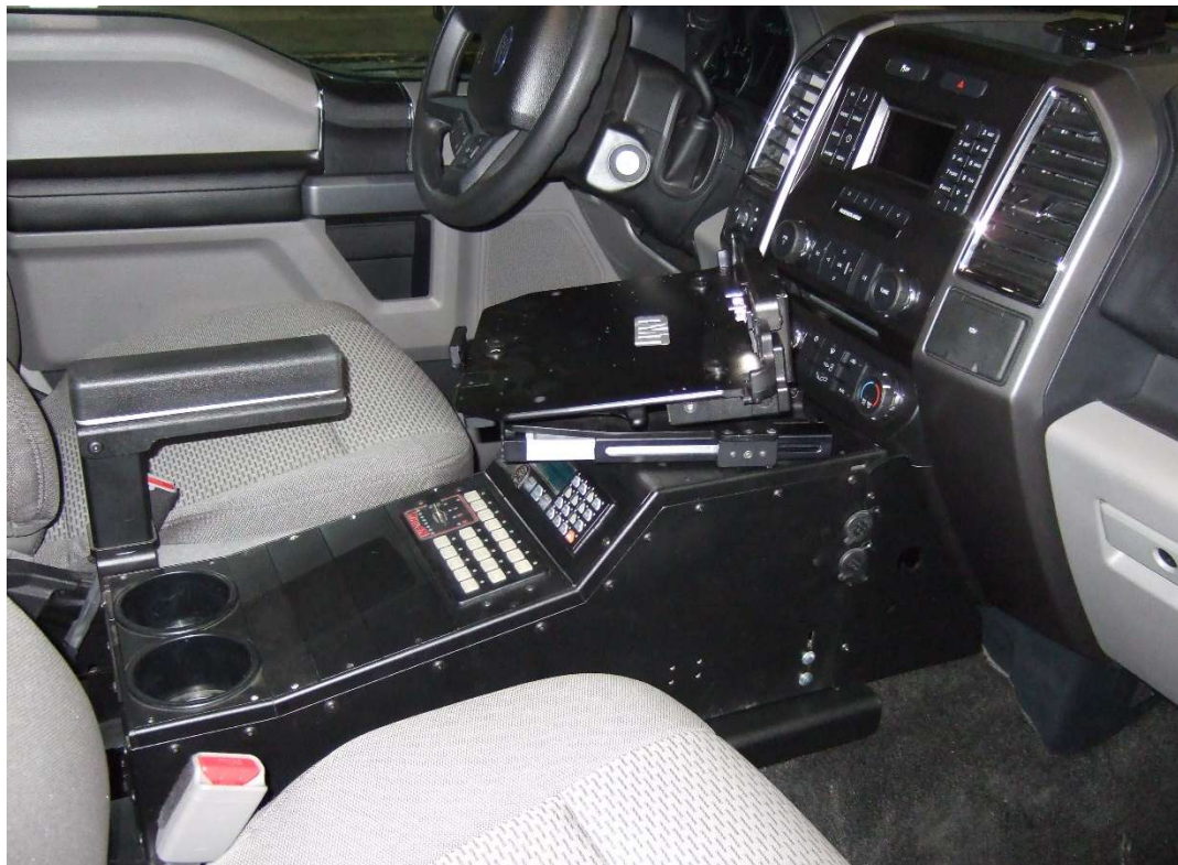
Standard 2015 F150 console with break-away armrest, trim panels, and Mousetrap Motion Mount
