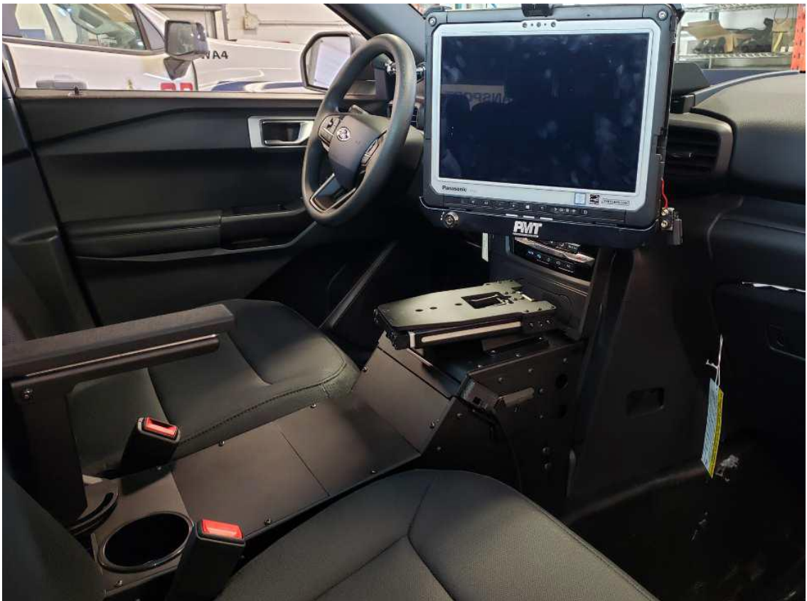
Interceptor utility printer in console with break-away armrest and Mousetrap Motion Mount
