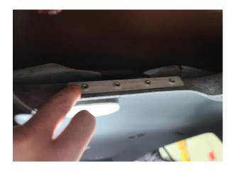
**Step 5**Put the headliner mount in place, and use #10-24x5/8 screws from the hardware bag to attach it
