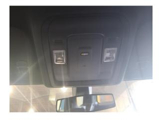
**Step 2**Gently use prying tools to OEM headliner, and remove the "T" shape cover
