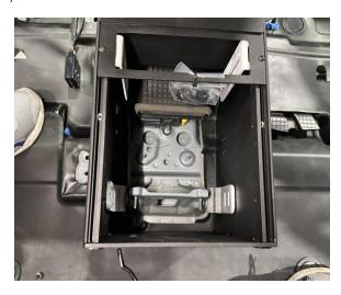
**Step 12**Align console shell and trim panels and then tighten all hardware.
