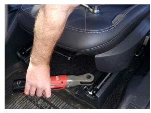
**Step 2**Remove OEM center console. PPV version shown.
