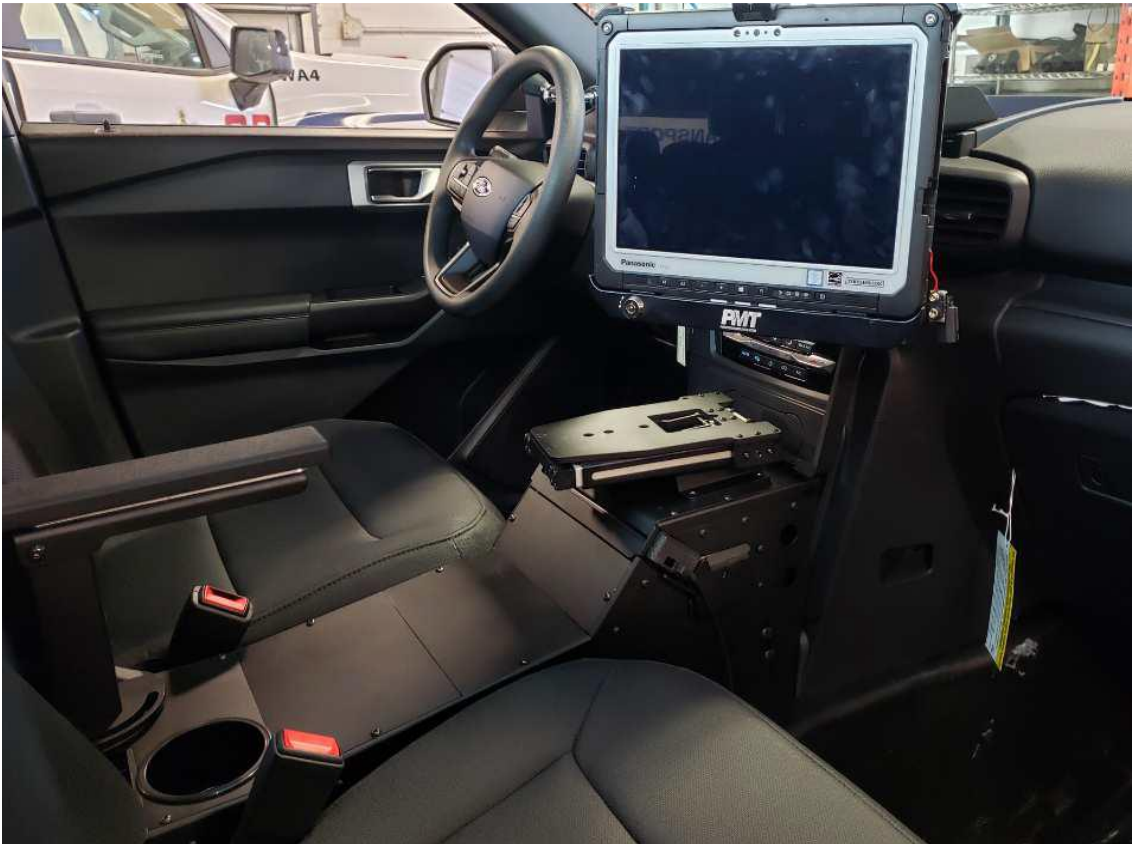
Interceptor utility printer in console with break-away armrest and Mousetrapp Motion Mount
