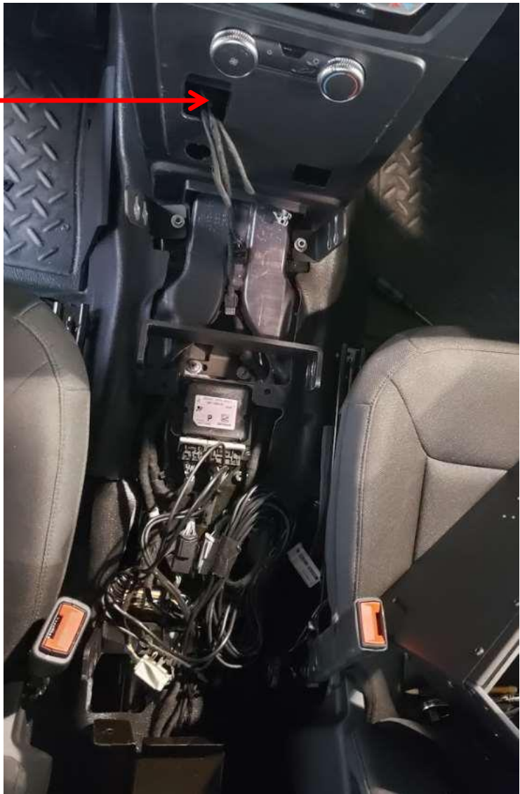
Console area picture after trimming
