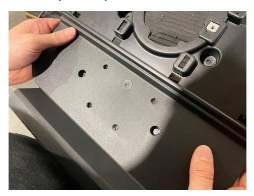
**Step 15:** Reinstall the plastic tray and check that all the drilled holes lineup with the under plate before re-engaging the clips on the plastic tray. If the holes do not visually line up, then lift the tray piece and adjust the forward/back and left/right position of the underplate by loosening the OEM bolts and sliding it to the desired direction. You can also check the alignment by attempting to thread a button head screw into the underplate through the plastic tray
