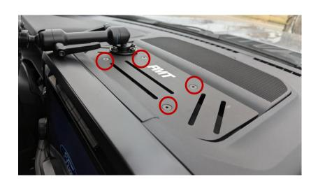
**Step 19:** Check the fit of the top mounting plate, if there is any interference you can change the position of the top plate by moving the top plate connector (middle component).
