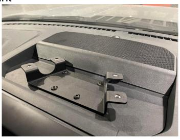
**Step 17:** Install all the mounts you want to have on your dash mount onto the top mounting plate in the position you want them (such as mobile device holders) these can be changed later with minimal disassembly. There are potential interferences with the top plate connector depending on the mount being installed onto the top plate. If there is interference, we recommend using buttonhead type screws with nuts and washers (pictured below)
