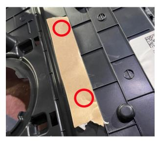
**Step 11:** Position the plastic tray panel in the dash as it would be installed and push down approximately where the screws in the under panel will be. Remove the underplate and remove the buttonhead screws, reinstall the underplate putting in all four OEM bolts
