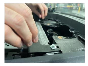
**Step 9:** Tighten the screws down so the plate will not move when pushed
