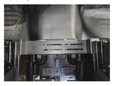
**Step 4**Slide the seat all the way to the front and place the Rear Leg such that the slots in the leg line-up with the seat bolt hole in the pedestal. See pictures below.
