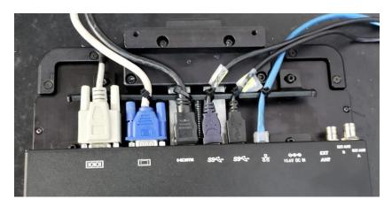
Connect all cables securely to dock ports, and use tie straps to secure cables to the "Cable Management Bar" as shown.
