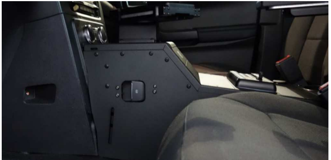
C. Push the console completely in, and make it aligned with the dash.
