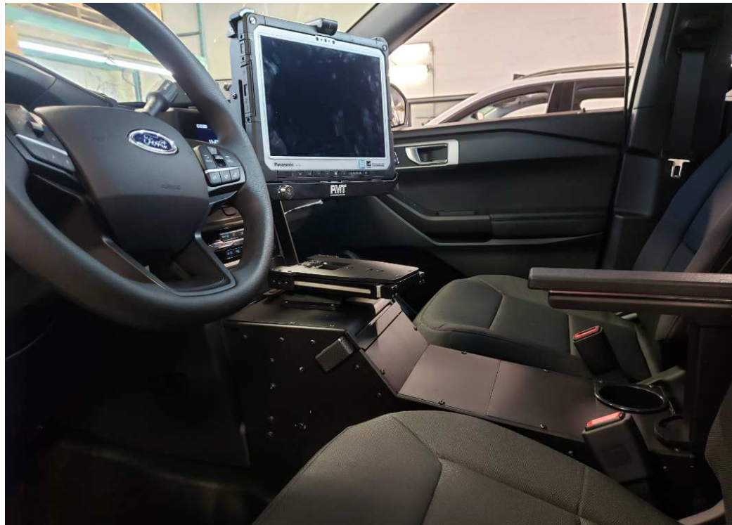
Standard Interceptor utility printer in console solution with break-away armrest and Mousetrap Motion Mount
