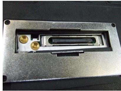
Once the door is fully open, inspect the connector for any pre-existing damage, that could then damage the dock. Do not proceed with docking if damage is present
