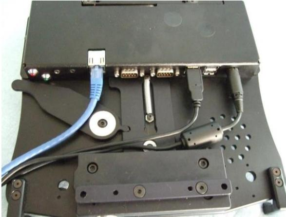
Securely connect required cables to matching ports, and use tie straps to secure cables to a suitable location on the dock to prevent cable strain
