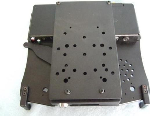
The standard mounting/interface plate that comes with the PMT TrimLine V series vehicle docks features industry standard mounting bolt patterns. This allows easy mounting to many pre-existing mounts as well as dedicated mounts from PMT
