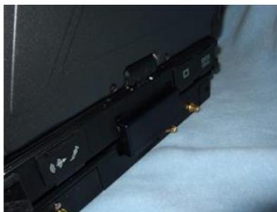
You should hear a click as the rear clamp springs forward, engaging into the rear of the computer
