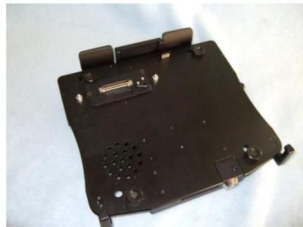
Our “Guide Plate” (part# 70.V100.014-1) optional accessory is great for use in environments where greater stress is placed on the docking connector due to rough handling, or awkward installations such as vertical walls. The plate works by adding additional locating surfaces that prevent mis-alignment and damaged dock connectors when inserting the laptop into the dock. Contact us to learn more, and to inquire about any of our additional accessories.
