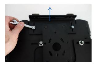
Step 3: With the cradle turned upside down, loosen the nuts for the depth adjustment bracket, and slide the bracket out
