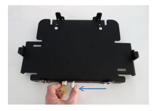
Step 1: Unlock cradle by turning key horizontal, then open cradle by squeezing the release handle towards the lock
