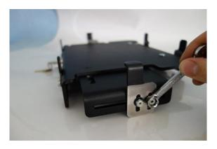
Step 2: Using a 3/8" wrench, loosen the nuts on the side and hold down clamps so they can move freely
