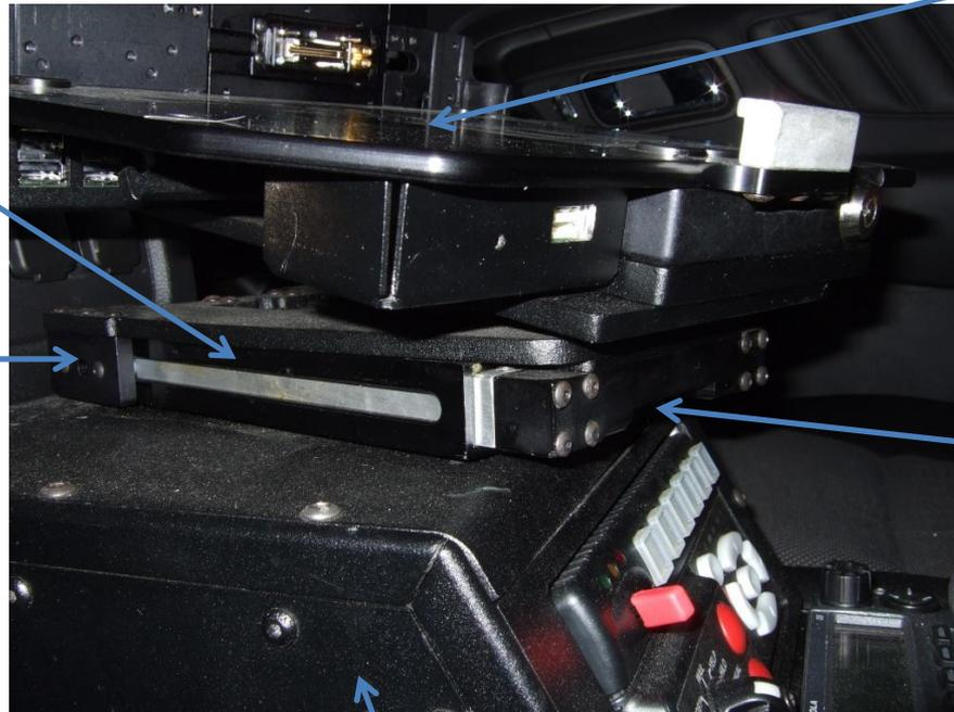
Slide release trigger (behind front pull handle)
