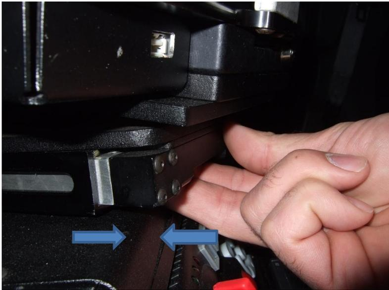
Squeeze release trigger
