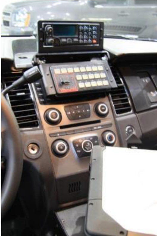
Unit is offset for gear selector clearance
