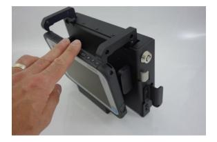
Step 2: Gently guide the tablet out of the docking station.
