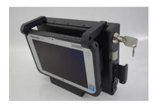
Step 4: For added security the dock can now be locked if so desired. Insert key, lock (rotate key to vertical), then remove the key.
