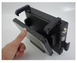
Step 2: Insert the computer bottom first and carefully align the computer onto the locating pins of the docking station.
