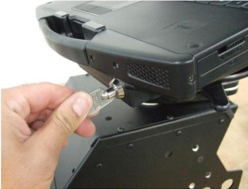
Step 1: Insert key and rotate 90 degrees counter clockwise. The docking lever will spring forward releasing the rear clamp
