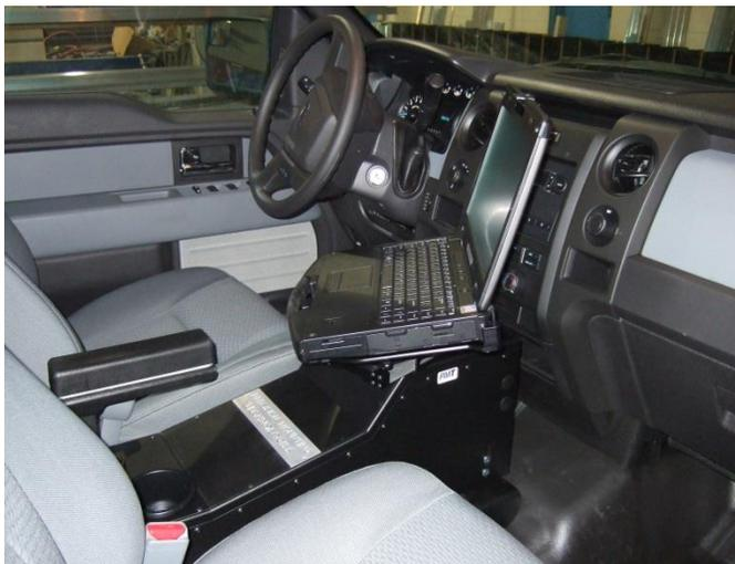
Photo shows SA-14 Vehicle Dock installed on PMT SightLine console in a 2013 Ford F150
