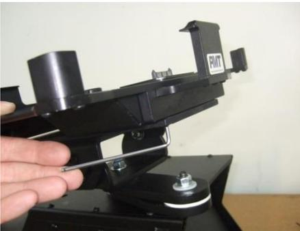
Next attach the dock (with cables already connected) to the interface plate using qty-4, 10-24 x 1/2" screws
