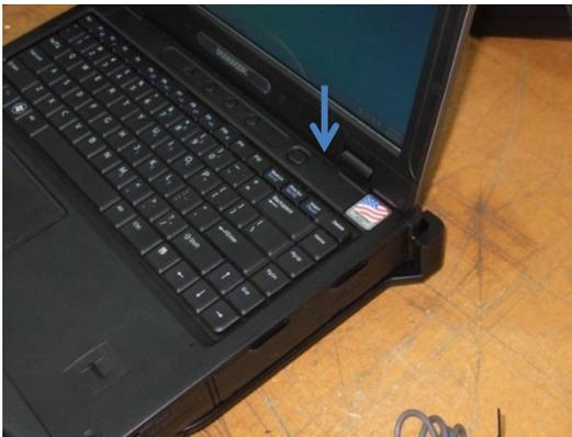
Step 3: Let the rear end of the computer down into the dock. A gentle push down is all that is necessary to ensure computer is fully seated.
