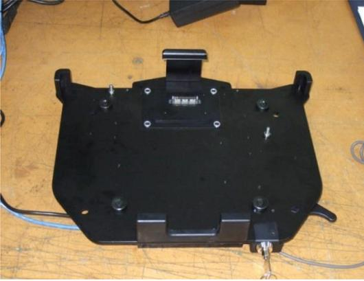
Step 1: Insert key and rotate 90 counter clockwise to prepare dock for computer. Note the docking lever springs forward and rear clamp slides back.
