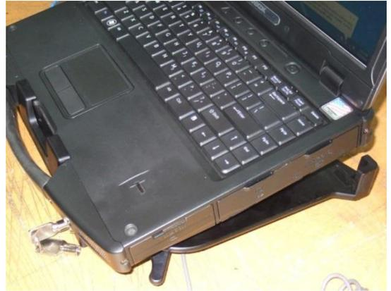
Step 2: Slide computer into dock front first so that front clamp grips computer in between handle.
