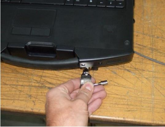
Step 5: While holding the lever back, rotate the key 90 degrees clockwise then remove the key.
