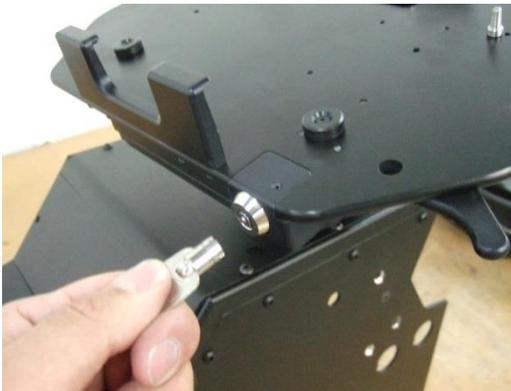
Step 3: You may now rotate the key 90 degrees clockwise and remove which will make re-insertion of the computer back into the dock quick and easy without needing to re insert the key
