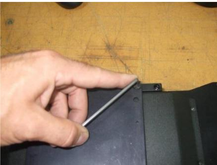
Tighten the 10-24 screws using an 1/8" allen key (hex wrench)
