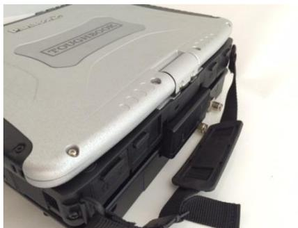
You should hear a click as the rear clamp springs forward and engages into the rear of the computer
