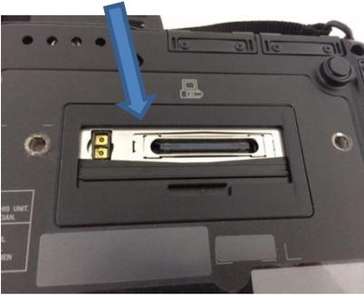
Turn the laptop over and ensure the connector cover door is fully open
