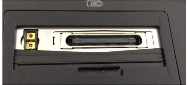
Once the door is fully open, inspect the connector for any pre-existing damage, that could then damage the dock. Do not proceed with docking if damage is present
