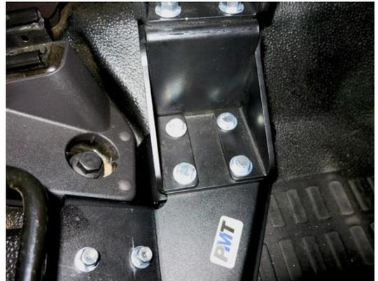
Step 6: Position the vertical pedestal , or offset riser (some vehicles may or may not require the Offset Riser) on the vehicle base and loosely thread the supplied hardware into the base. Fully tighten bolts once all four are installed
