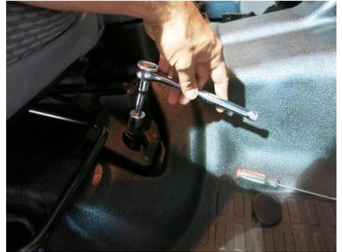
Step 2: Remove front seat mounting bolts completely
