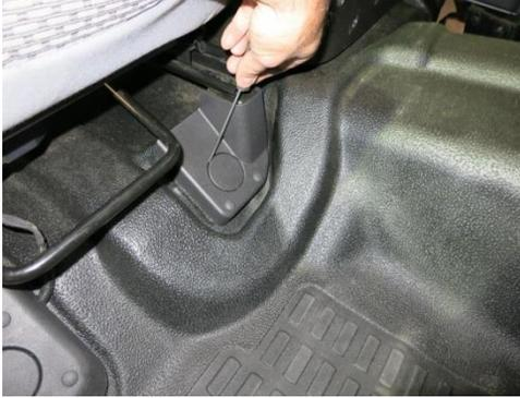
Step 1: Remove any plastic caps covering the front and rear seat mounting bolts of the front passenger seat
