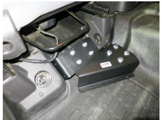
Step 4: Tilt the seat back, and slide the vehicle specific base assembly in between the vehicle floor and seat brackets. Leave any bolts present on vehicle specific base present, but loose.
