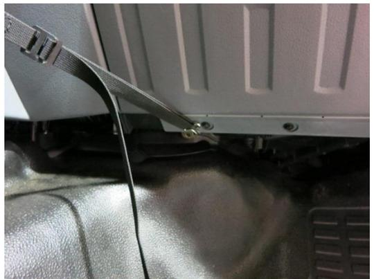
Step 8: Find a suitable location with steel bracing to hook the support straps into. Most vehicles have steel bracing behind the plastic panels under the glove box. Be sure that the area you chose to hook the straps is strong enough to support the load
