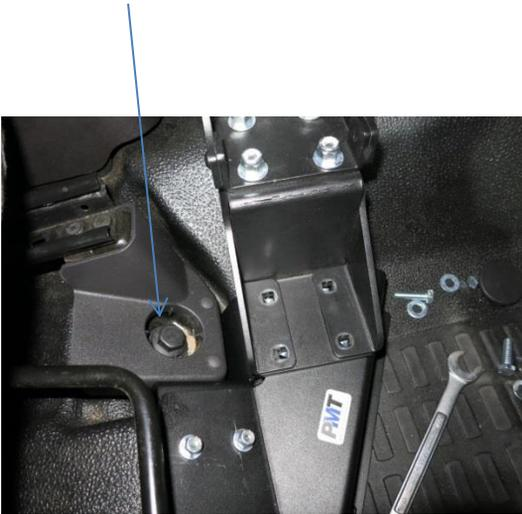
Step 5: Re-install the front seat mounting bolts and tighten to manufacturers specified torque. Re-tighten rear bolts to specified torque as well.
