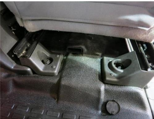
Step 3: Loosen, but do not remove the rear seat mounting bolts
