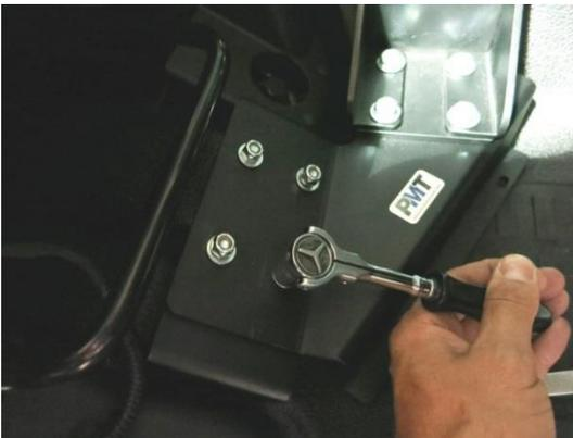
Step 7: If present, tighten alignment bolts on vehicle base
